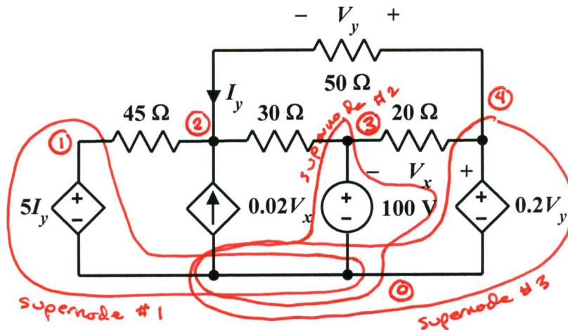
$$V_1 = 5 I_y \quad (\text{constraint equation for supernode } \#1)$$
